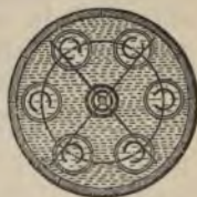
Fig. 84.—Arrangement for electrotyping all surfaces at once.
